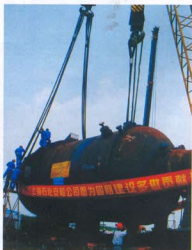
FOUR LEG WIRE ROPE SLING with main ring & sub ring at one end hooks at other ends
